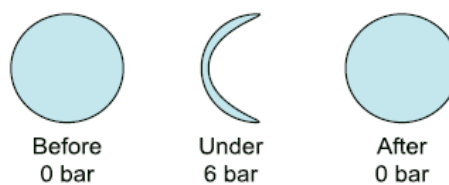
Figure 3.4 Deformation of microballoon under hydrostatic stress
