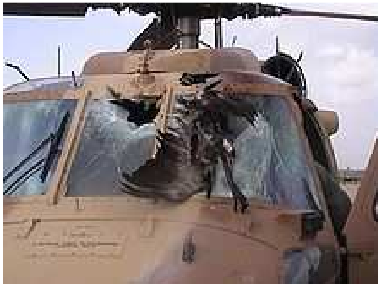
Figure 1.4. A UH-60 Black Hawk after a collision with a common crane, and the resulting failure of the windshield [5]
