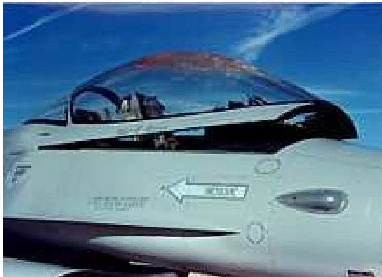
Figure 1.2. F-16 canopy after a bird strike [3]
