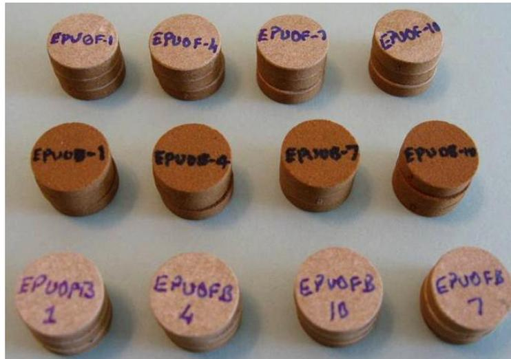
**Figure 5.29. 0-PU Coated Eco-Core Specimens**
