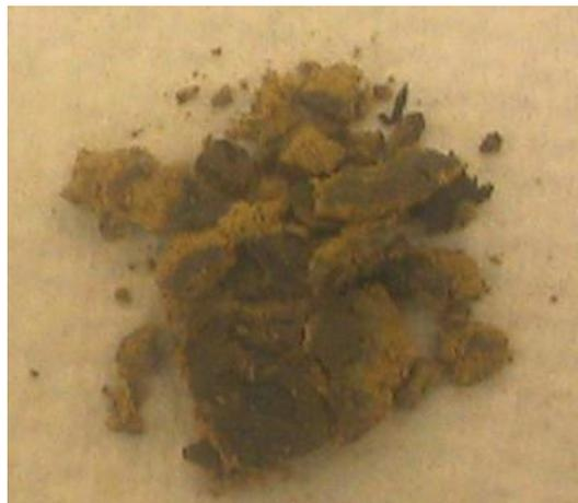
**Figure 5.69. Impregnated Eco-Core Specimen after Dynamic Testing**
