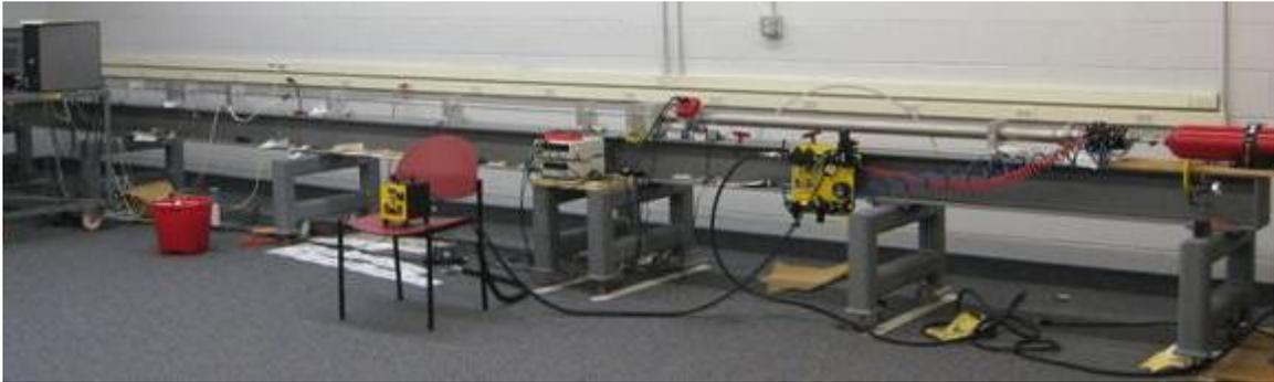
**Figure 4.4. Photograph of SHPB Test Apparatus**
