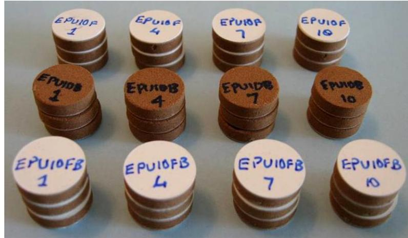
**Figure 5.30. 10-PU Coated Eco-Core Specimens**
