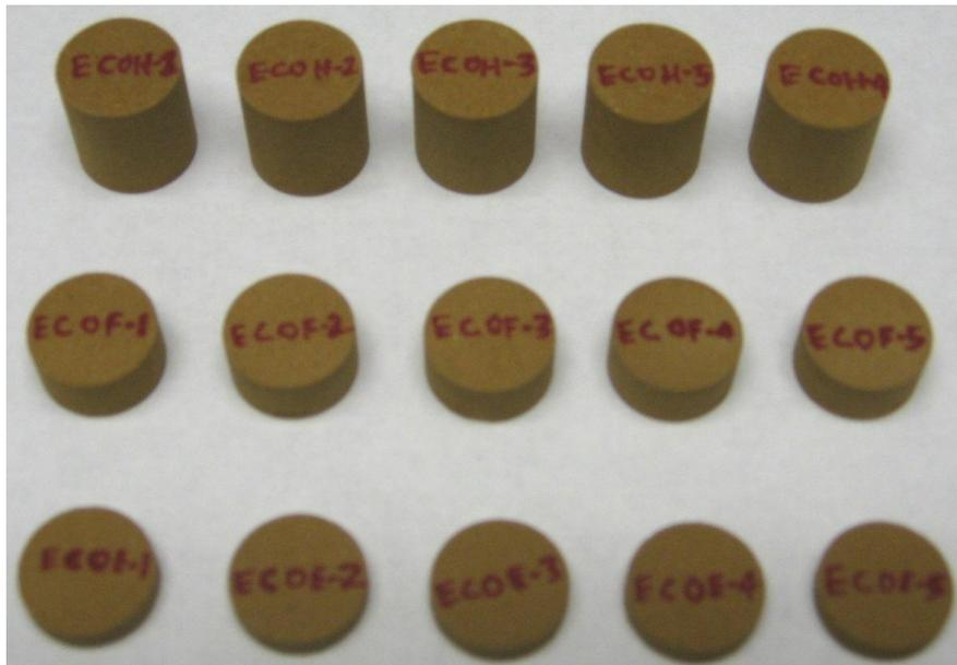
**Figure 5.1. Eco-Core Specimens of Various L/D Ratio's**
