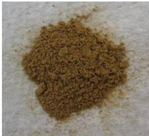
**Figure 5.6 Eco-Core Specimen after Dynamic Testing**
