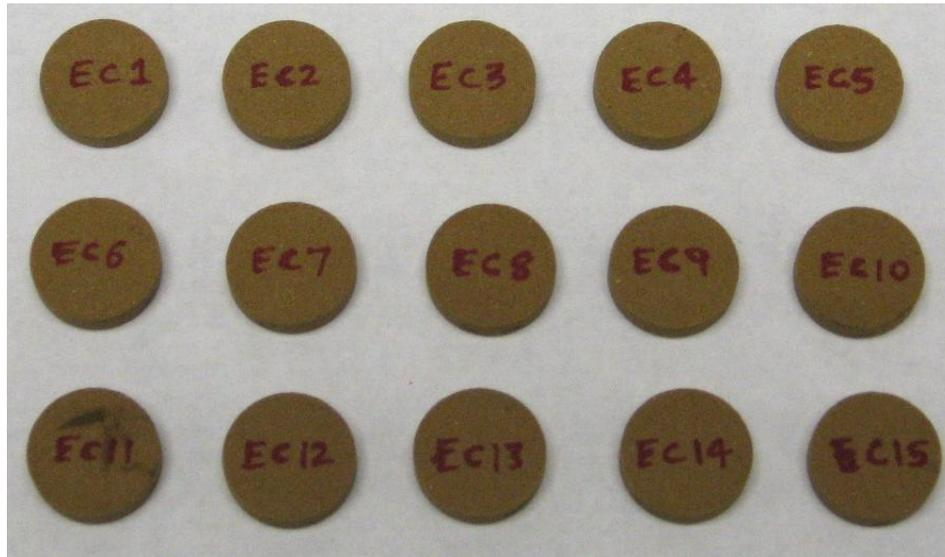
**Figure 5.2. Eco-Core Specimens for Dynamic Failure Model Development**
