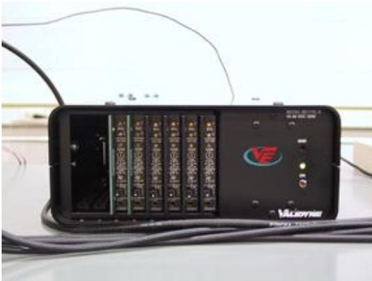
**Figure 4.14. Strain Gage Signal Conditioner**
