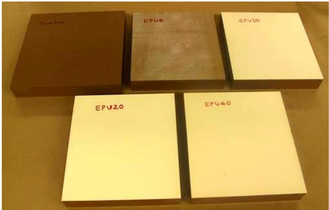
**Figure 3.3. Photograph of Polyurea Coated Eco-Core Panels**
