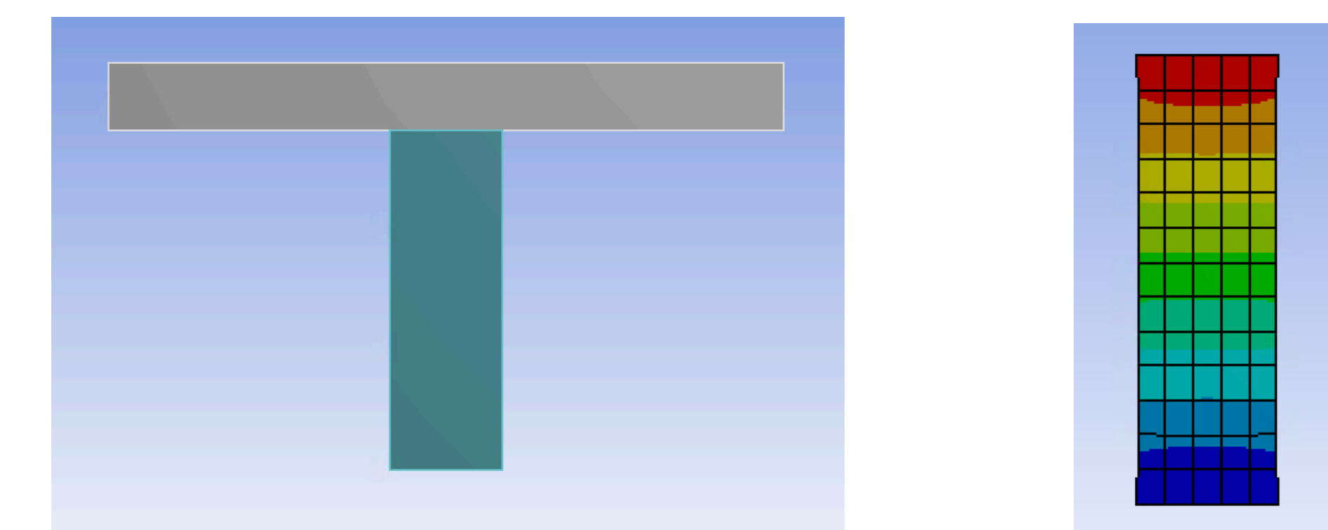
Figure 3. Left: Model of the tensile test set-up prior to deformation. Right: Model of the rectangular specimen after deformation.
