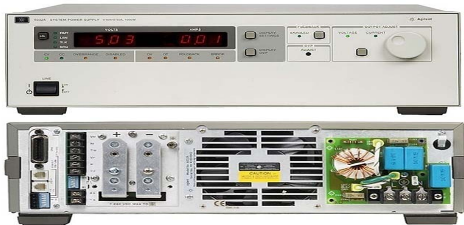
Figure 3.6. Agilent 6030A programmable power supply (front and rear view)
