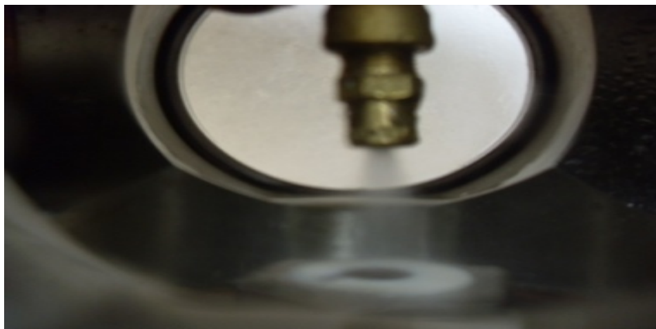
Figure 3.5. Fluid impingement on a test surface
