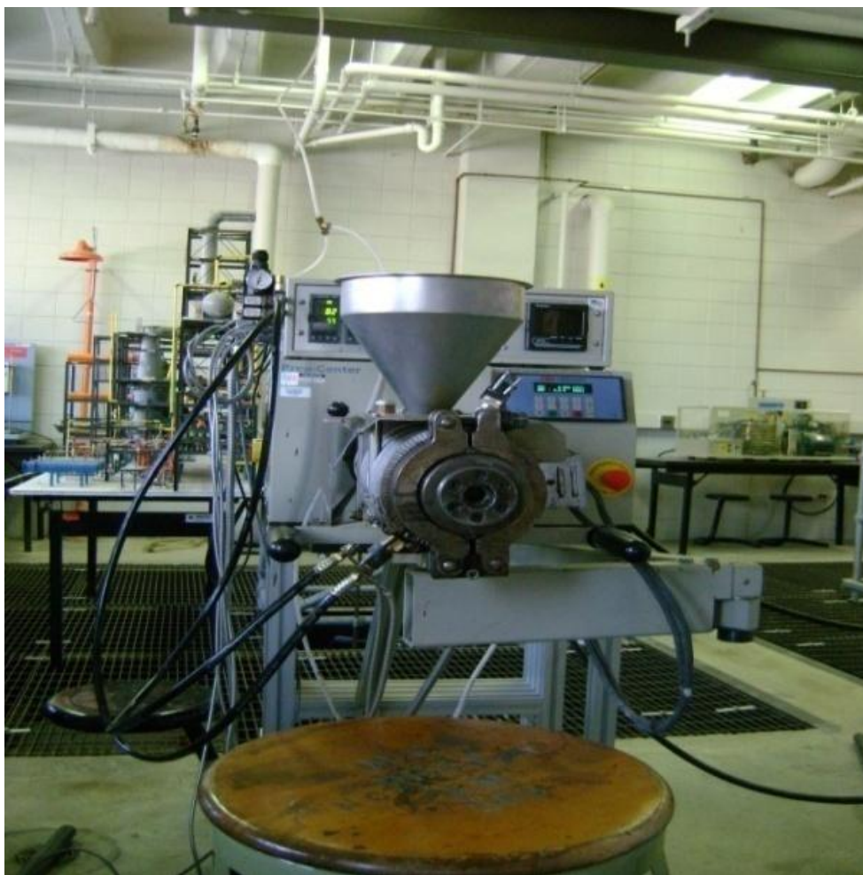
Figure 3.2 Twin Screw Mixer, (C.W. Brabender Instruments, Inc)
