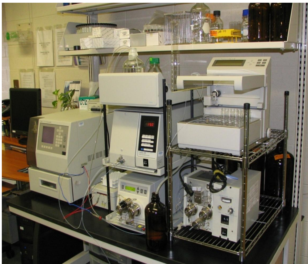
Figure 3.5 High Pressure Liquid Chromatography HPLC (Waters, Milford, MA)
