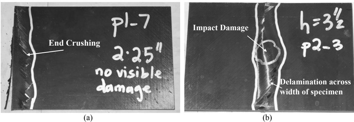
Figure 5.9. Failure modes of interleaved laminates. (a) Edge-crushing failure and (b) Failure at the impacted site
