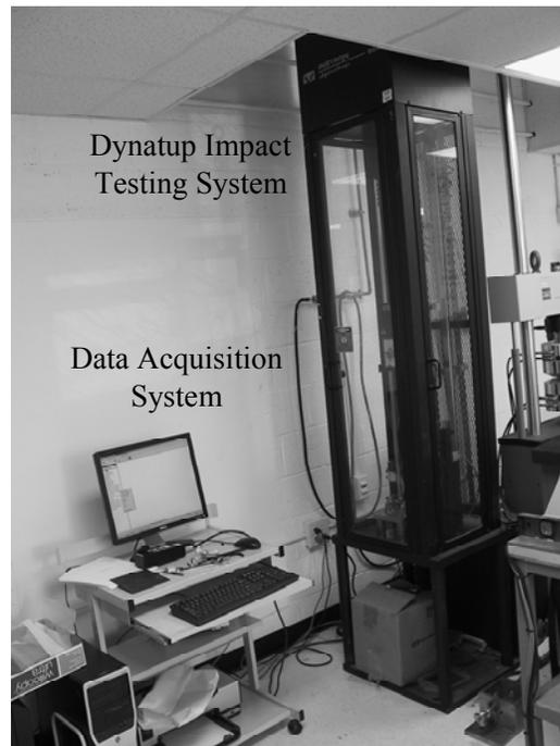
**Figure 4.1. Photograph of the Dynatup Model 8250 Impact Testing System and data acquisition system**
