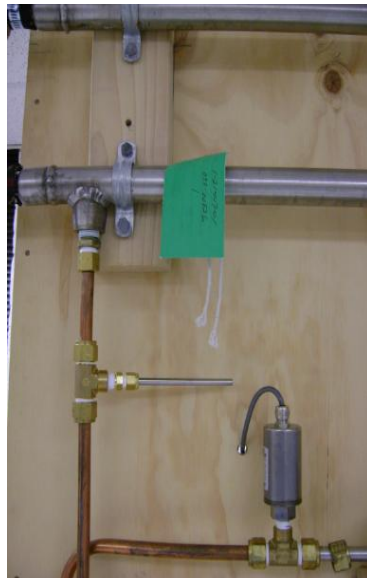
Figure 3.24: Photograph of one of the thermowells used in the present study.
