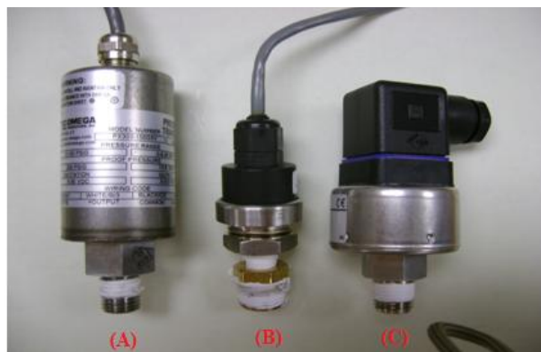
Figure 3.25: Photograph of the pressure transducers. (A) PX303-100GV, (B) PX480A-300GV, and (C) WIKA model ECO-1.
