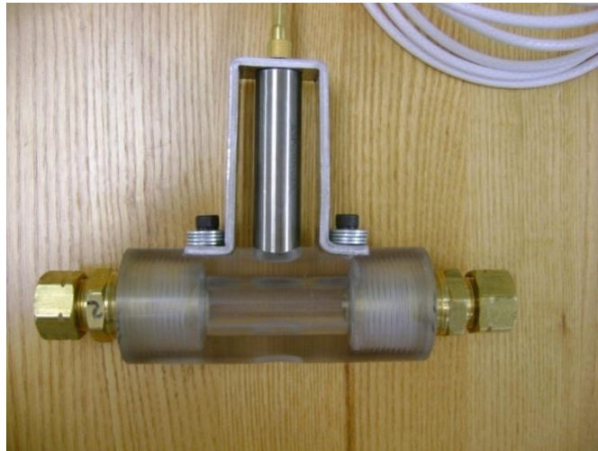
Figure 3.32: Photograph of void fraction sensor Design A used in the present study.
