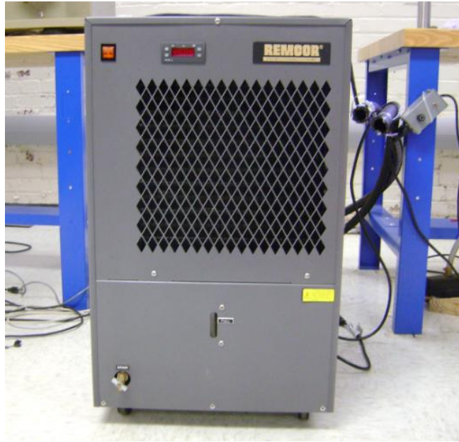
Figure 3.8: Photograph of the Cornelius REMCOR CH750-A series chiller used in the present study.
