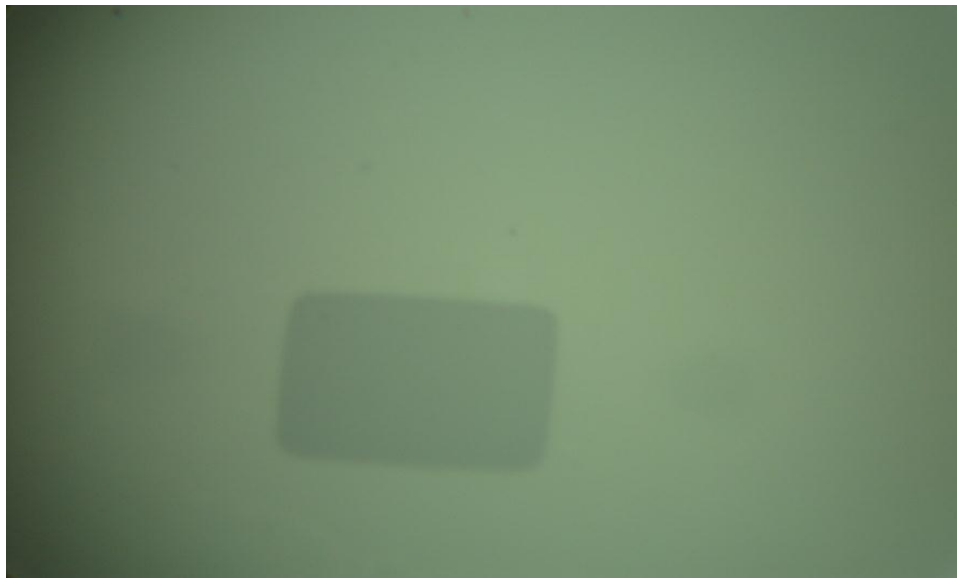
Figure 4.15. Effect of excessive etching on the fabrication of TFTs
