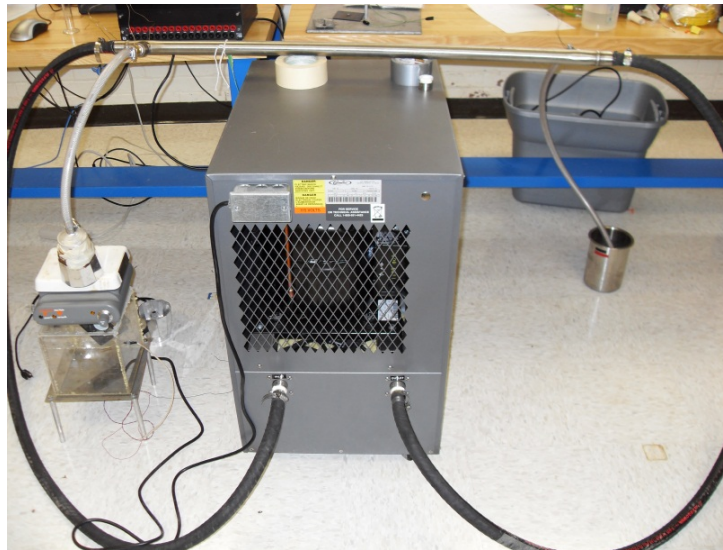
Figure 3.33. Actual heat exchanger and chiller test
