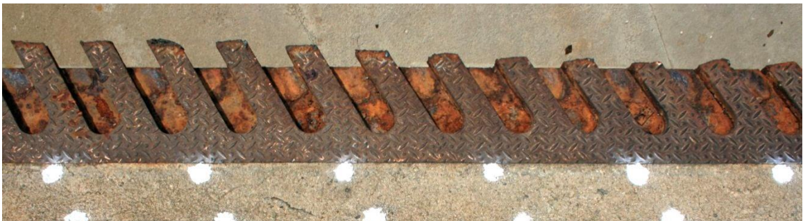
Figure 2.2. The finger joint used in this study. The empty spaces between fingers accommodate the fingers for the opposing half of the joint, which has been removed.
