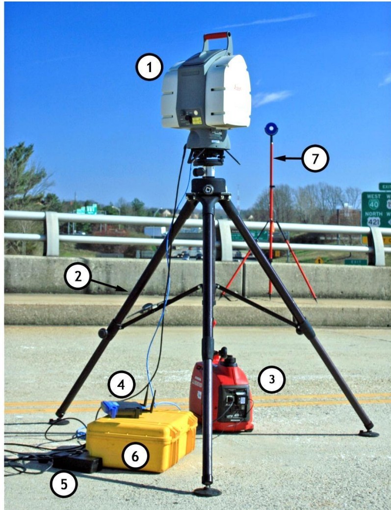
Figure 3.2. The Leica ScanStation.
