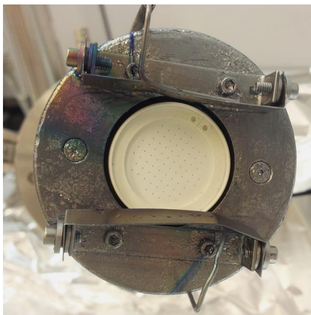
Figure 26 RF plasma source deflector plates and aperture disc
