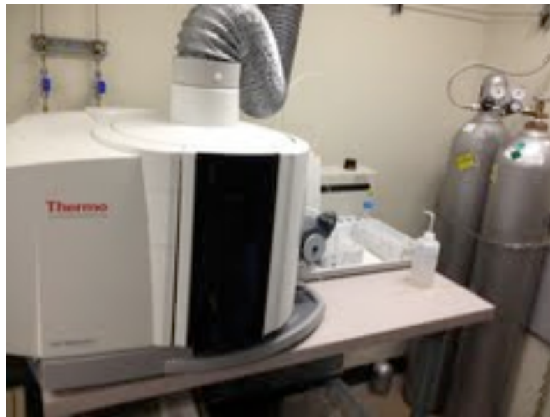
Figure 3.16 Depiction of inductively coupled plasma equipment
