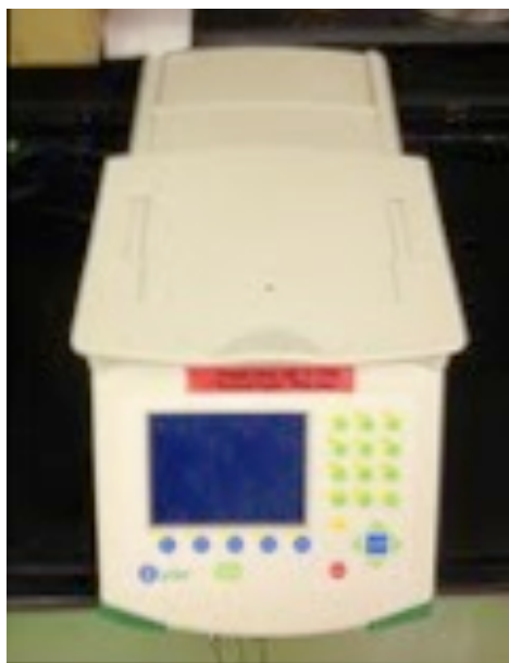
Figure 3.18 Depiction of iCycler thermo cycler from BIO-RAD
