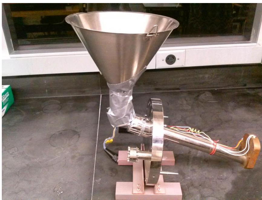
Figure 3.9. Liquid N 2 substrate holder
