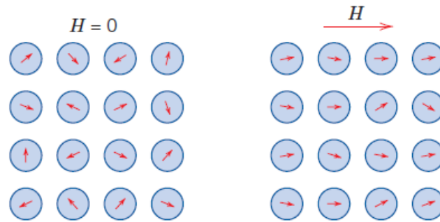
Figure 2.3. The paramagnetic behavior of atomic dipoles due to an applied magnetic field [13]
