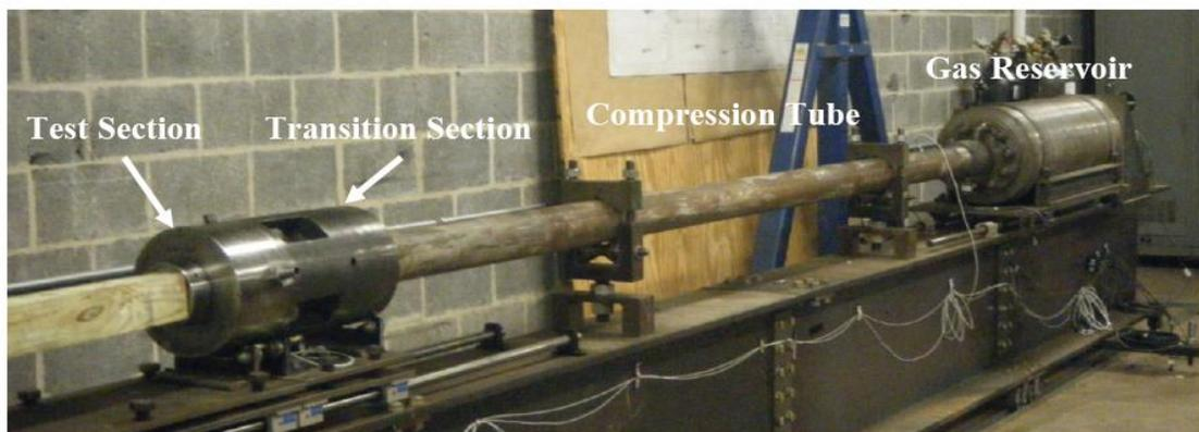
**Figure 2.8 120 kpsi ballistic compressor at PSU [Sirignano, 2011]**
