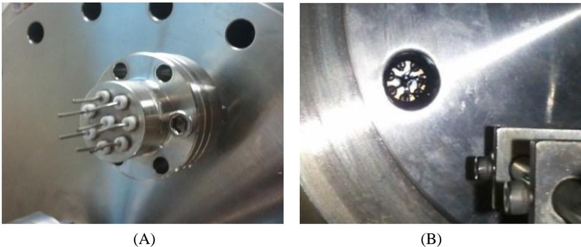
**Figure 3.3 (A) Electrical pin feed-through outside chamber, (B) Feed-through inside chamber**
