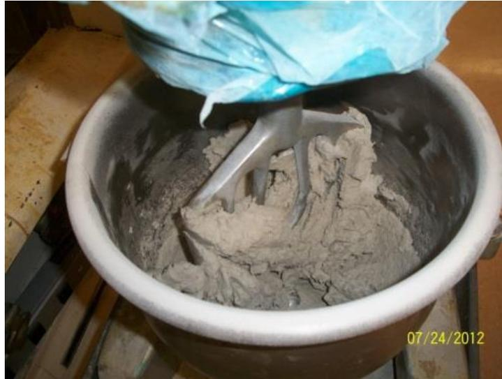
*Figure 2.2.* Fly ash-resin mixing process.
