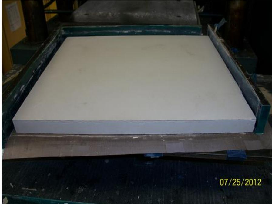
Figure 2.5. Photograph of cured Eco-Core panel.
