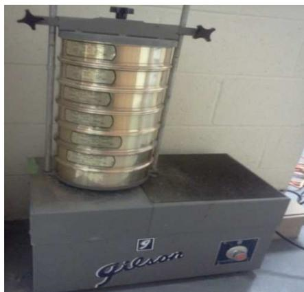
*Figure 12.* Sieve size arrangement and shaker for particle size analysis
