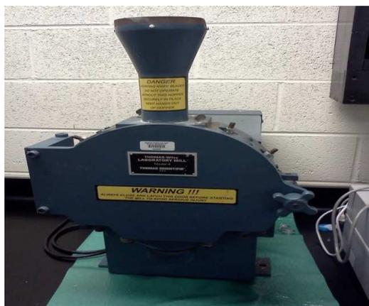
*Figure 10.* Thomas Wiley Mill for grinding MSW samples
