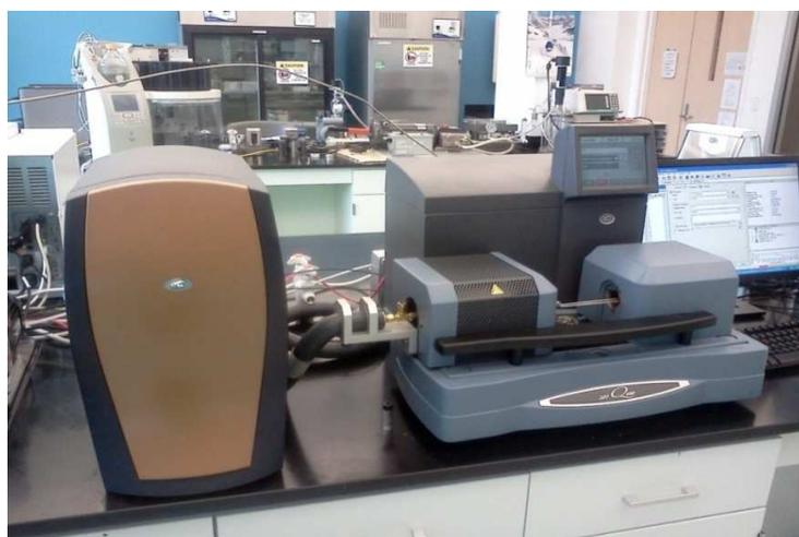
*Figure 17.* Thermo gravimetric- Differential Scanning Calorimetric- Mass spectrometry (TGA-DSC-MS) analyzer (TA Instrument)
