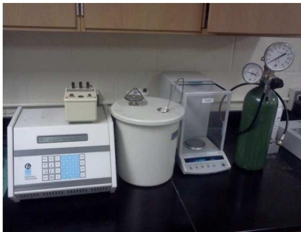
*Figure 14.* Oxygen Bomb calorimeter for heating value determination
