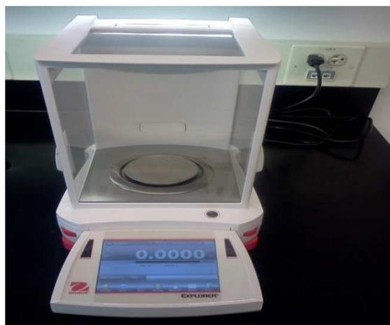
*Figure 13.* Measuring balance for weighing MSW samples and products
