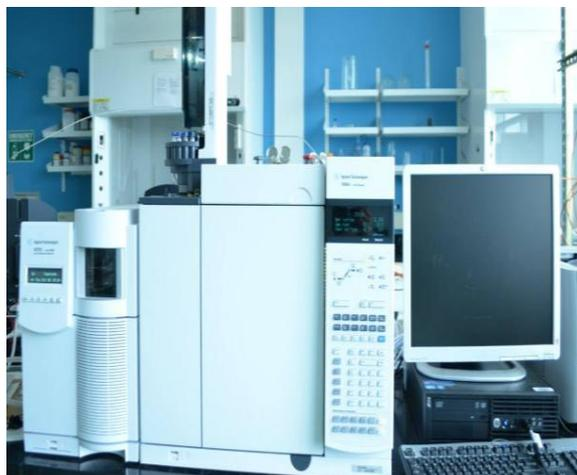
*Figure 21.* GCMS used to analyze the oil extracted from microalgae
