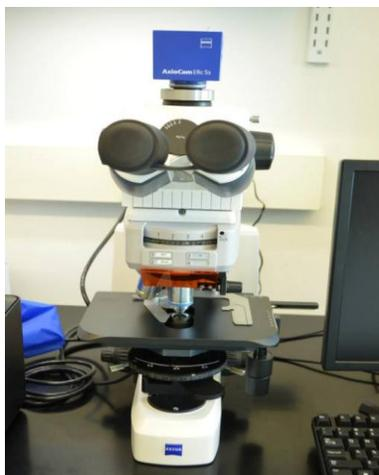
*Figure 17.* Zeiss microscope used to check the bacterial or fungal contamination.
