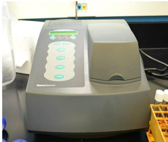
*Figure 13.* Spectrophotometer used to measure the optical density at 680 nm spectrum.
