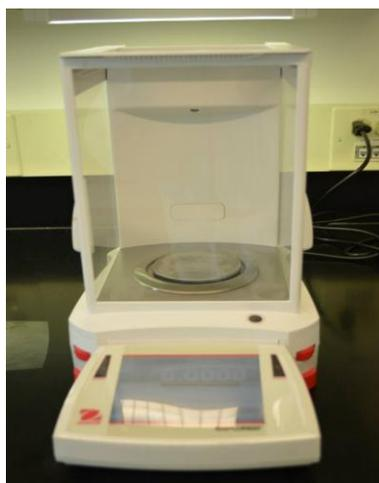
*Figure 18.* The electronic balance.
