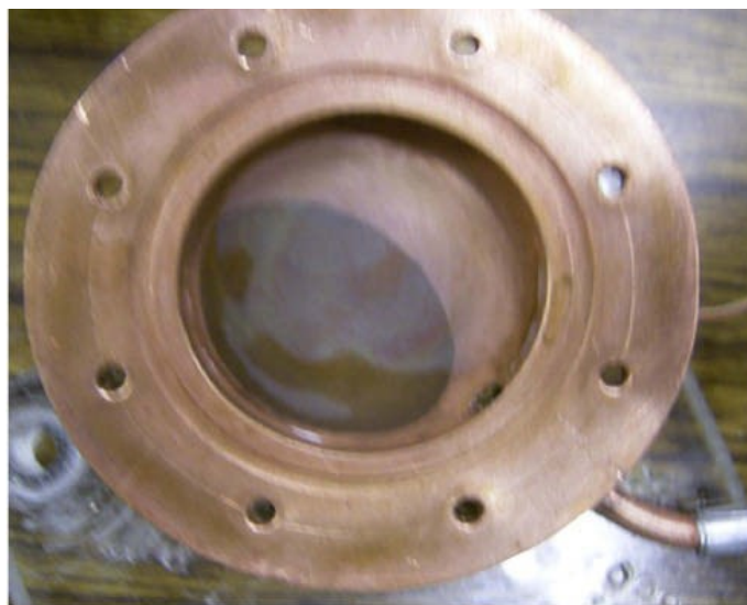
Figure 22. Oxidation of the container inside the compensation chamber (Singh et al., 2010)
