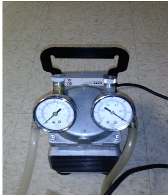
Figure 45. Vacuum pump for charging system
