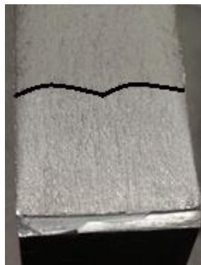
Figure 19. Outlined crack face of thick specimen
