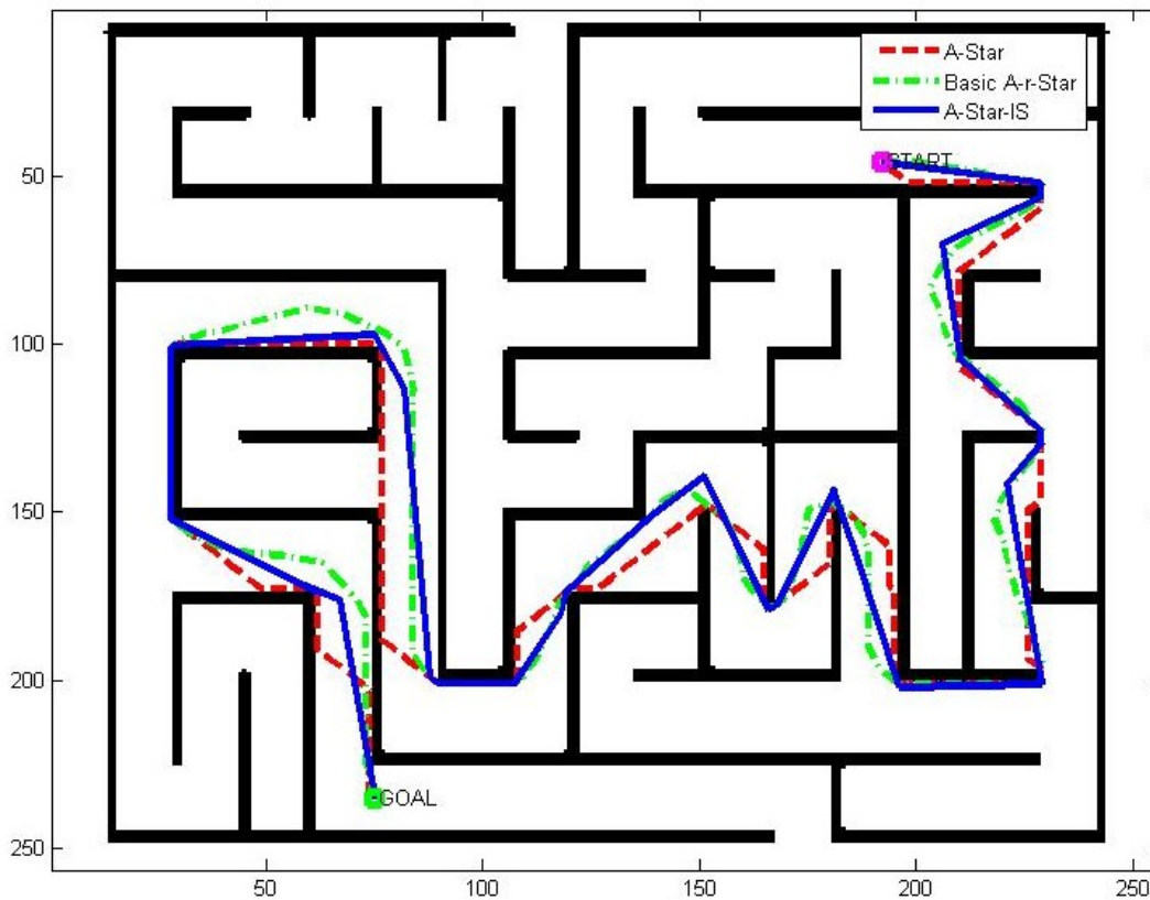
Figure 5.17. How A-Star, Basic A-Star and A-r-Star operating on a uniform grid world solves a maze problem.
