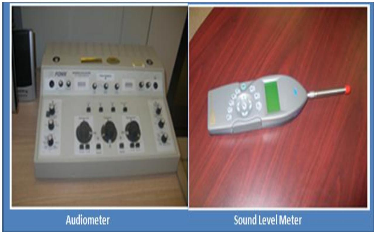
*Figure 4.* Audiometer and sound level meter.
