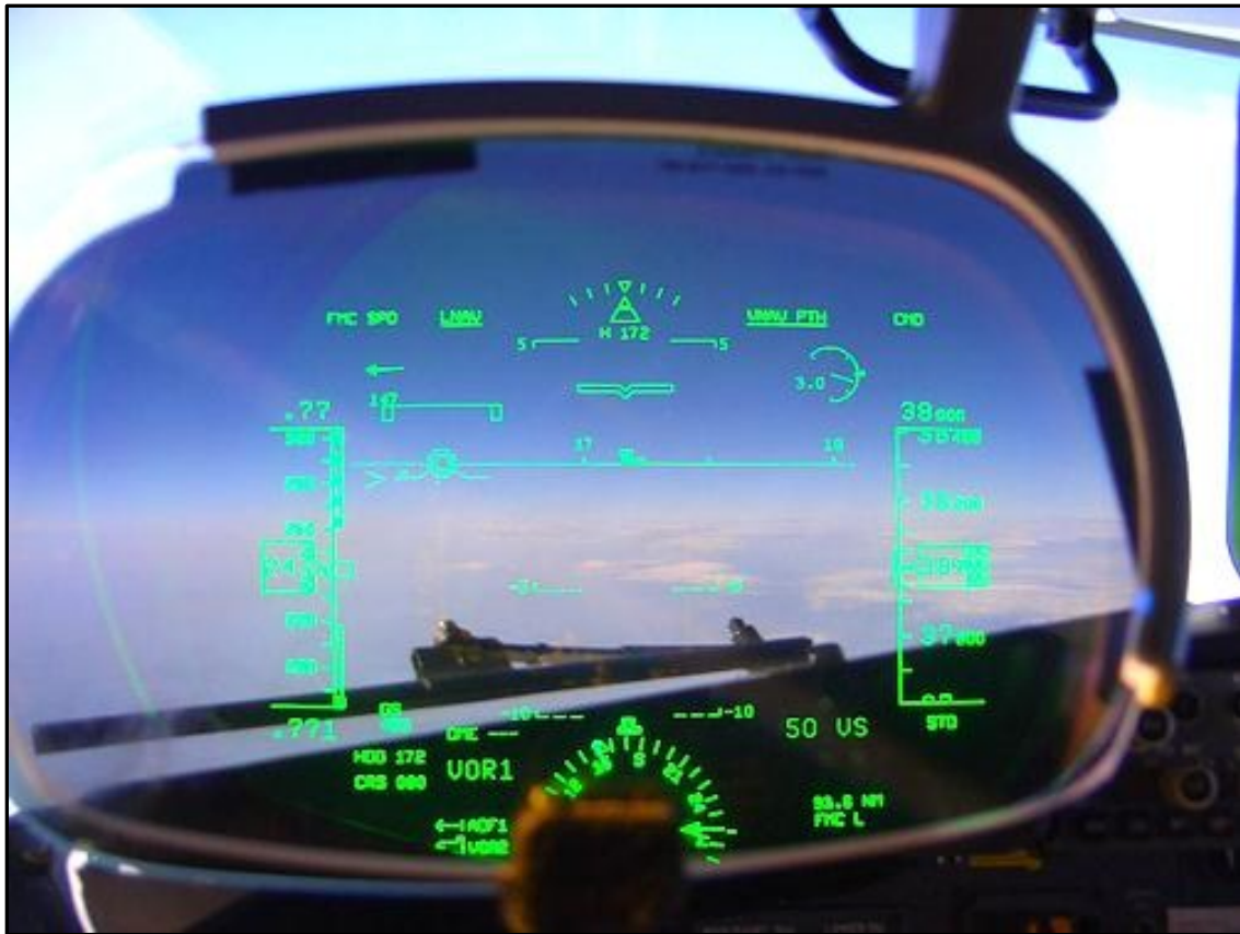
Figure 4.6. Heads-up display – aviation.
