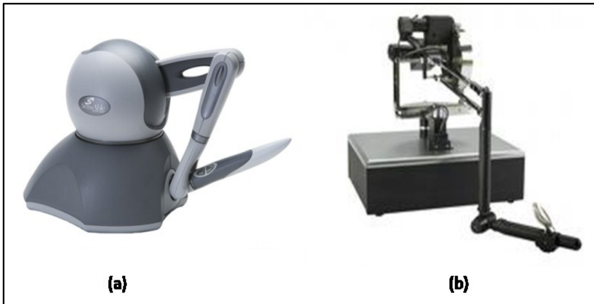
Figure 4.7. Sensable™ haptic controls: (a) Phantom Omni; (b) Phantom Premium.
