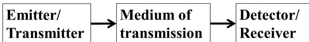
Figure 1.3. Block diagram of a typical infrared device application.
