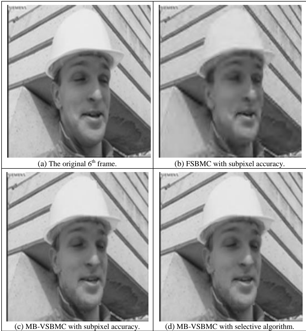
Figure 4.7 The comparison of the compressed 6 th frame for “Foreman” sequence using three different block partitioning techniques.
