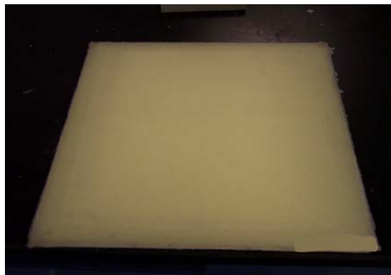
Figure 4.7. Cured prepreg 12 in. x 12 in. with electrospinning treatment
