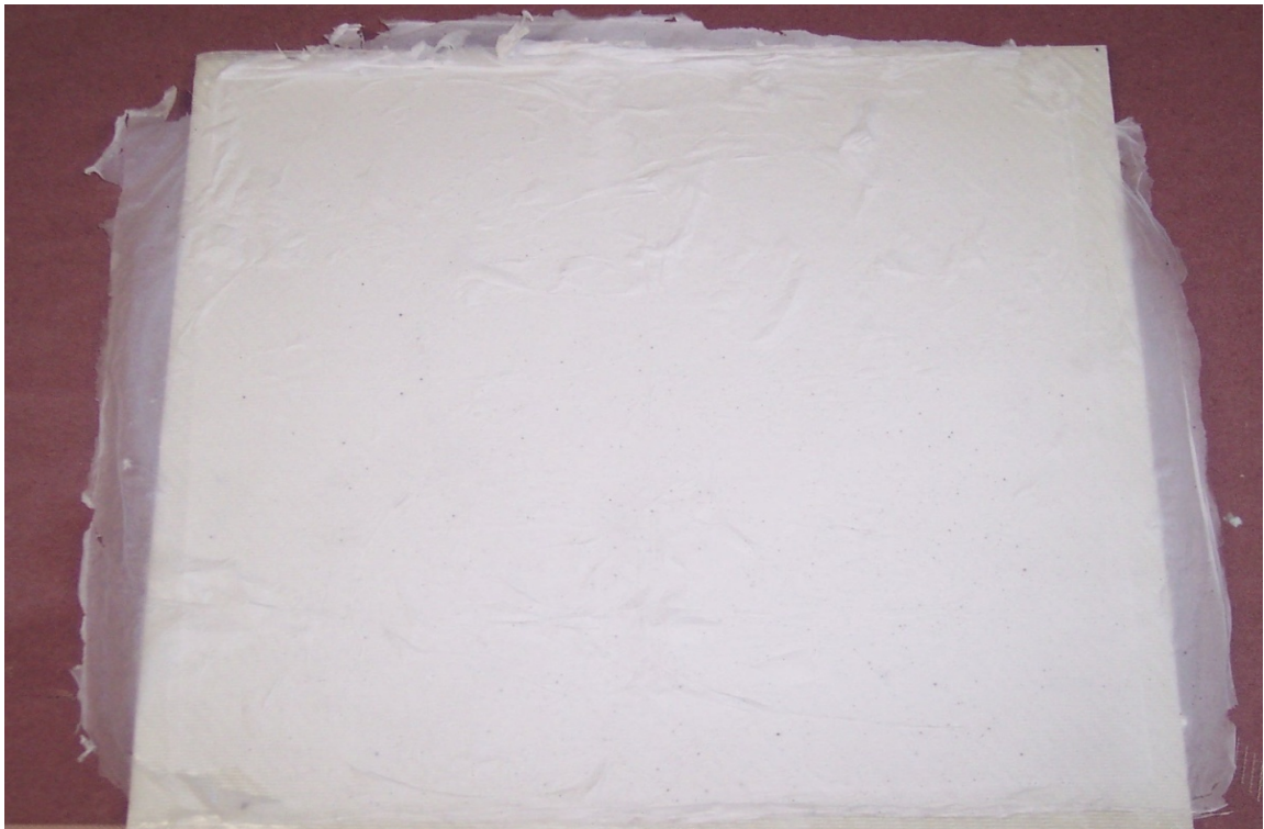
Figure 4.6. Picture of application of electrospun sheet to interface
