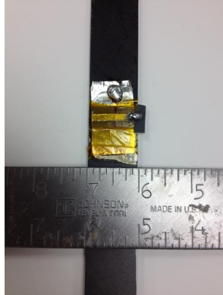
Figure 3.2. Bonded PZT sensors on CFRP specimen.
