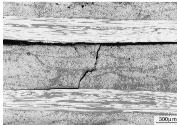
Figure 2.10. Matrix cracking and delamination (Diao et al., 1997).
