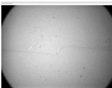
Figure 4.2. EBL field stitching error
