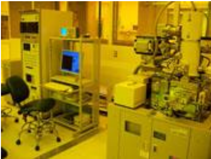
Figure 4.1. Elionix ELS-7500 EX E-Beam Lithography System [66]
