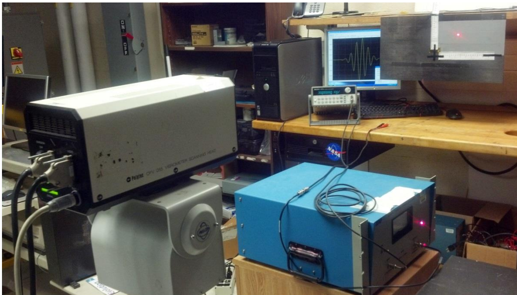
Figure 13. Actual SLV scan in progress.
