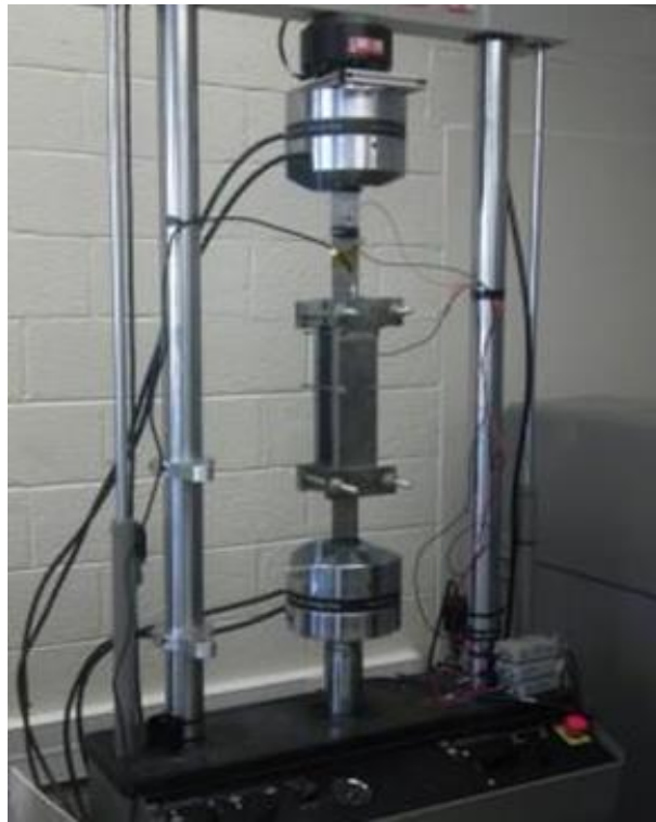
Figure 3.6. MTS machine with test assembly
