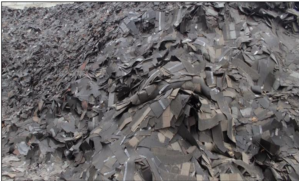
Figure 2.3 Tear-off shingles after service life
