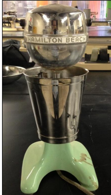
Figure 3.1 A typical grinder used to prepare the tear-off shingles
