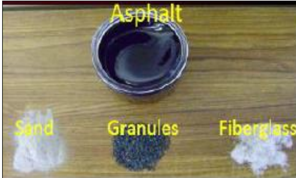
Figure 2.4 Composition of asphalt shingles (from Grzybowski, 2010)
