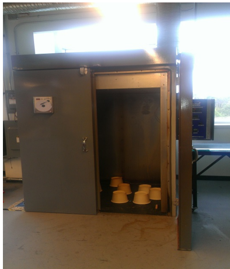
Figure 2.12. LR Technologies ST867TUL240V90KW walk in oven used for curing cycle of the composite fabrication
