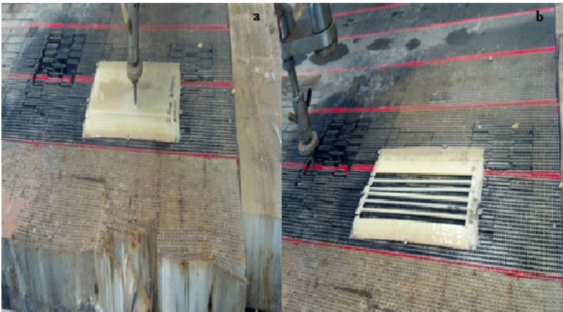
Figure 3.2. Water Jet machine for cutting the flexural coupons
