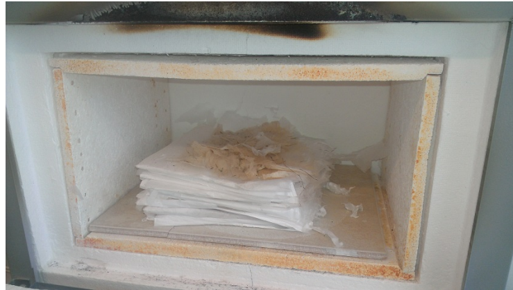
Figure 2.6. TEOS electrospun nanofibers folded, stacked, and sintered at 600 degrees C
