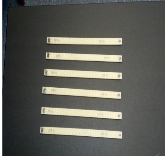
Figure 3.4. S2 fiberglass flexural coupons with sintered TEOS electrospun nanofibers numbered
