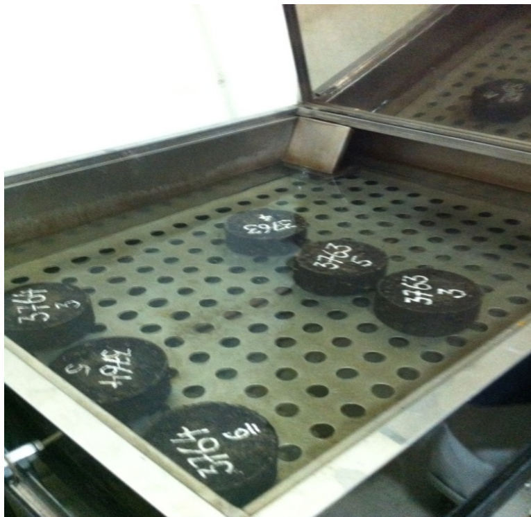
Figure 3-2. Asphalt Mixture Sample Replicates
