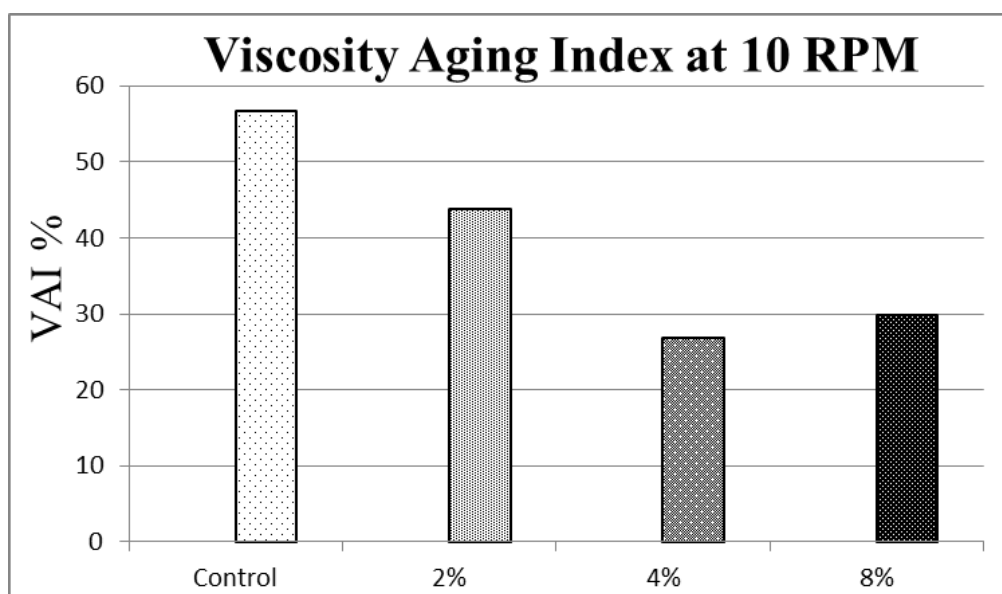
Figure 5-9. Viscosity Aging Index of Binders After Short-term Aging at 10 rpm
