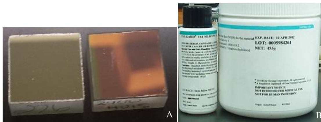
Figure 4.1 (a) Picture of optical diffraction gratings with groove densities of 1200 lines/mm (left) and 2400 lines/mm (right). (b) PDMS kit used to duplicate pattern from optical diffraction grating and produce elastomer stamp.
