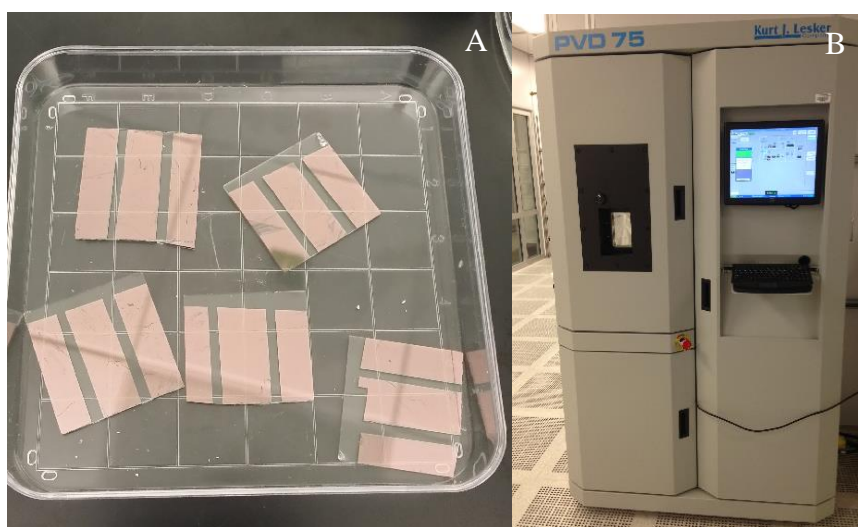
Figure 4.3 (a) Substrates with gaps in between gold coated area. (b) Physical Vapor Deposition machine used to coat substrates in conductive metal.
