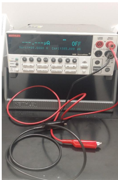
Figure 4.4 Source meter used to measure current and source voltage.
