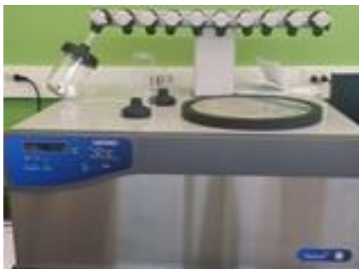
Figure 4.6 Lyophilizer used to vacuum moisture from sample.
