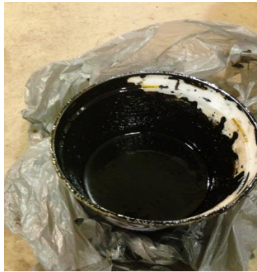
Figure 3.2 Bio-binder produced at NCA&T Farm
