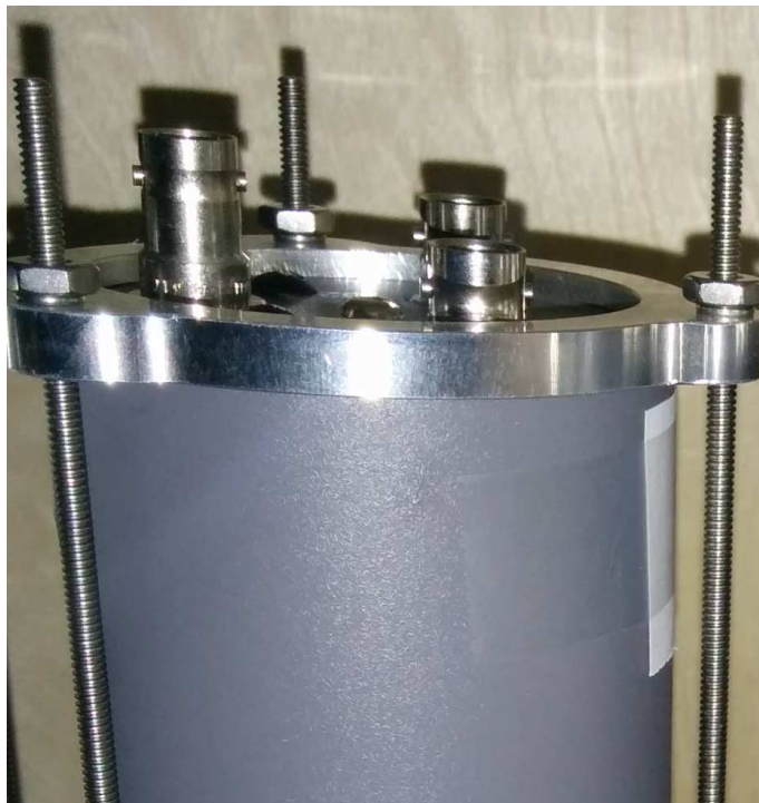
Figure 4.5: View after the three threaded rods have been tightened the back brace securing the PMT to the quartz bar
