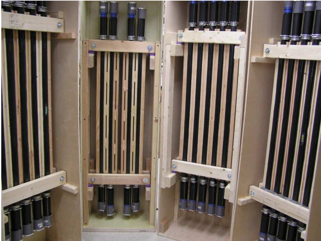
Figure 4.6: All 4 wooden crates and racks filled with quartz bars waiting transport to JLab
