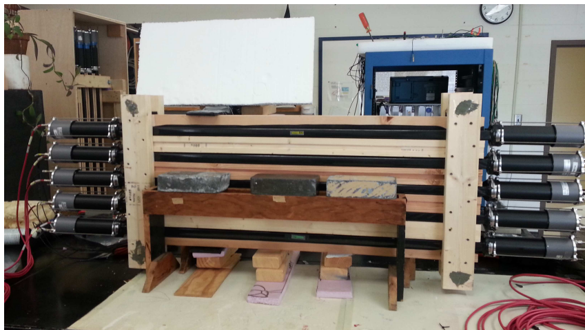
Figure 5.1: Setup for cosmic ray testing
