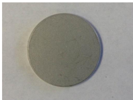
Figure 9. Membrane support (MPSS 316 L disc).
