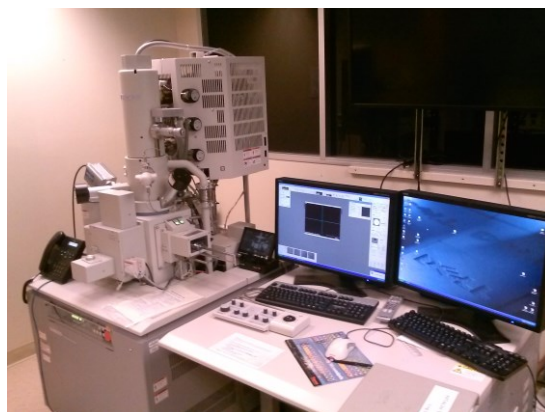
Figure 11. HITACHI-SU8000 Scanning Electron Microscopy
