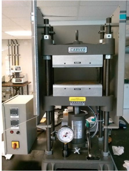
Figure 7. The lab hydraulic press with digital heated platens.
