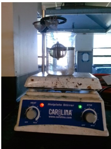
Figure 8. Hotplate stirrer with magnetic field
