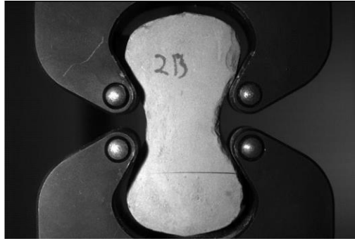
Figure 4.22. View of Briquette F.2 with the Crack Propagated through the Briquette
