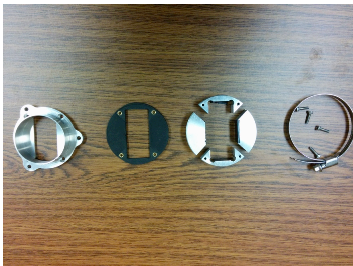
Figure 4.3 PMT brace components
