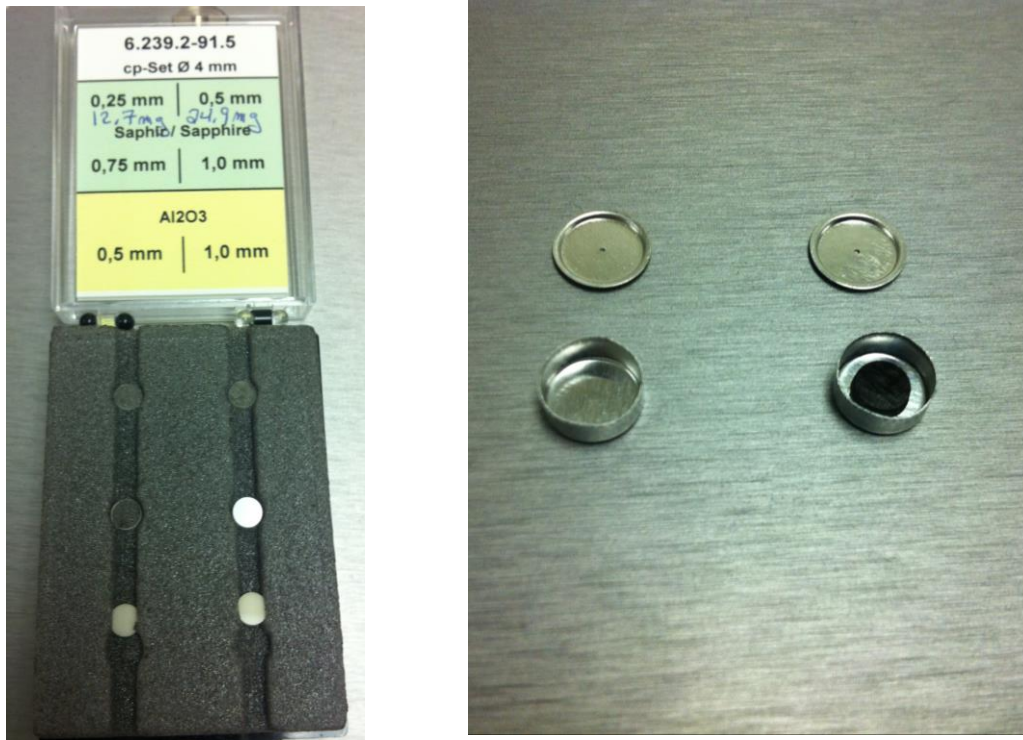
Figure 4.8 The Sapphire and IM7-G/8552 with pans and lids
