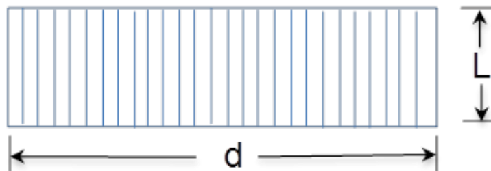
Figure 3.5 Specimen model of thermal diffusivity axial direction samples
