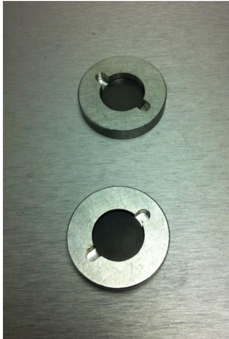
Figure 4.2 The FlashLine™ 2000 specimen holders and specimens
