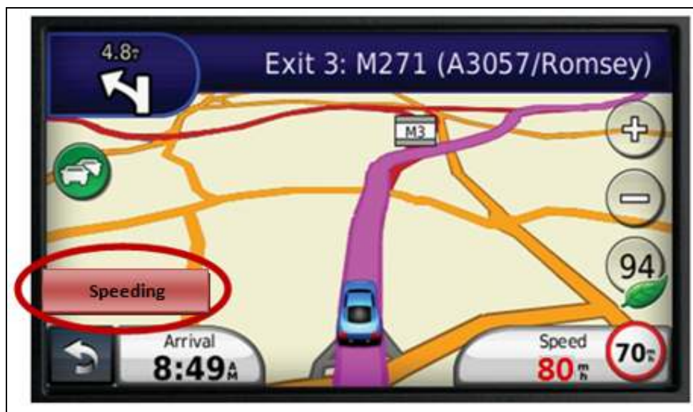
Figure 3.6. GPS Speed Alerting Features.
