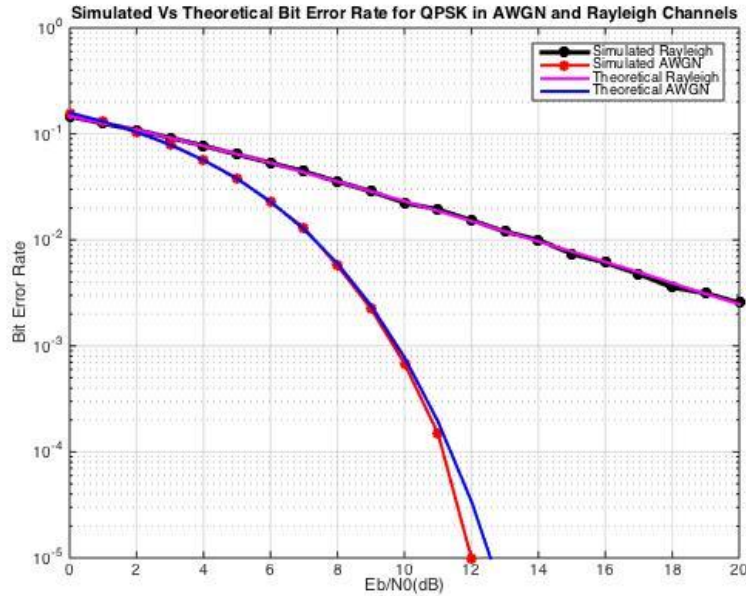
Figure 19. Performance of DS-CDMA QPSK modulation in AWGN & Rayleigh environment.
