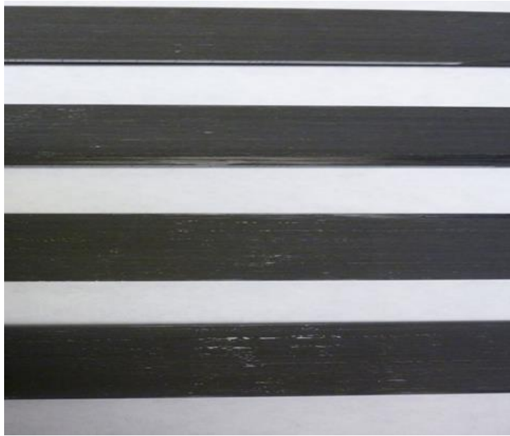
Figure 3.1 AS4/3501-6 composite prepreg for laminates fabrication
