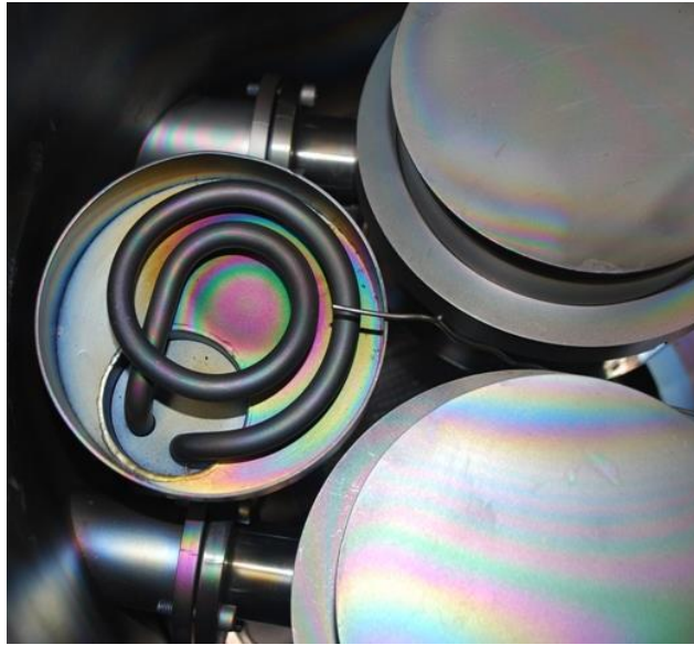
Figure 6. Radiant heater used for ET deposition.
