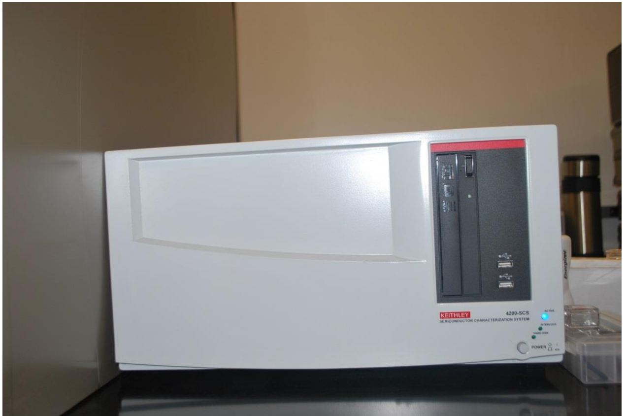
Figure 12. Keithley 4200-S system used for current-voltage measurements.
