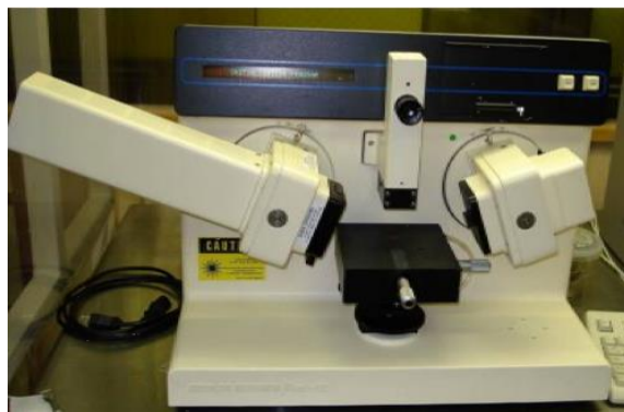
Figure 11. Rudolph Research Auto EL II Ellipsometer.
