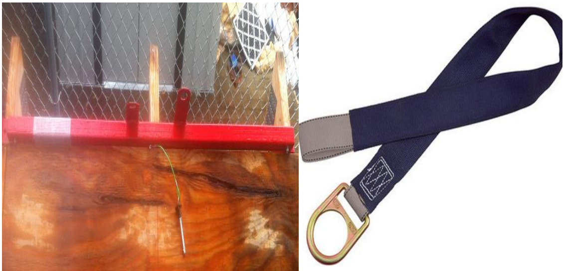
Figure 13: Metal braced and tie-off anchorage
