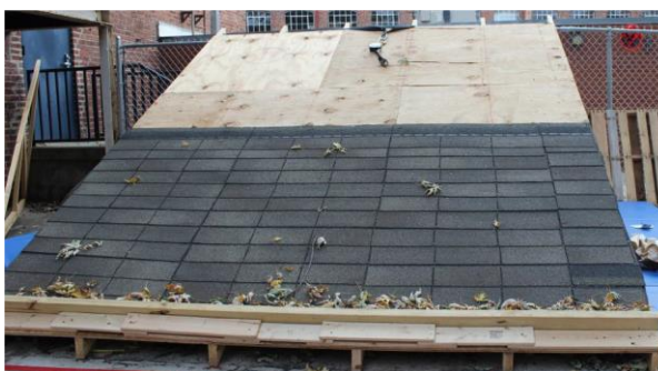
Figure 10: Indoor and Outdoor scaled models used for the study.
