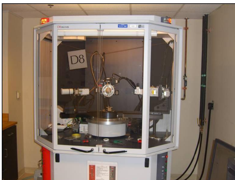
Figure 3.9. Diagram of NC A&T x-ray diffraction.
