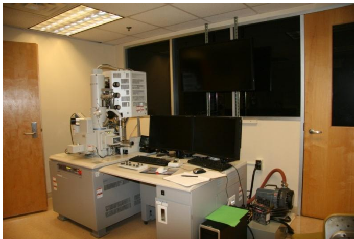
Figure 3.6. Hitachi SU8000 Field Emission Scanning Electron Microscope.
