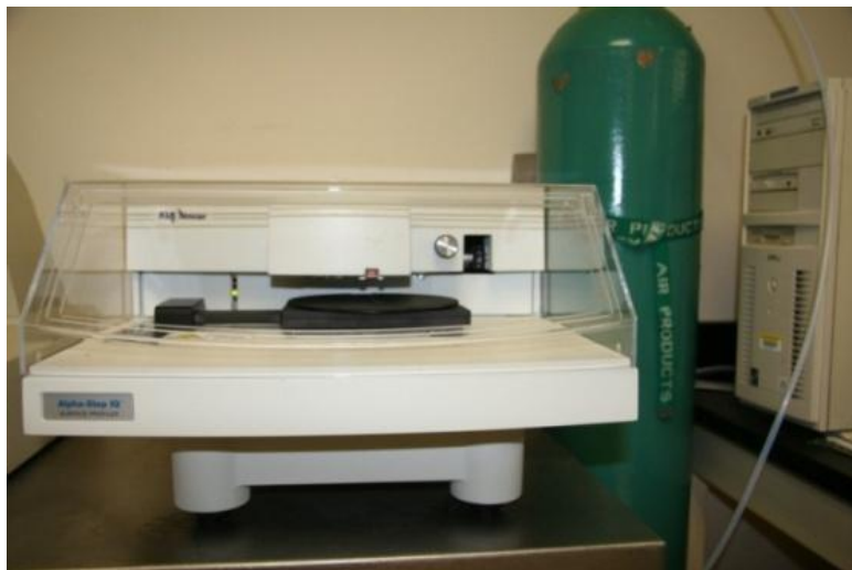
Figure 3.4. Diagram of profilometer used.
