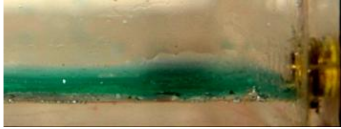
Figure 44. At the entrance of fuel line water domain pinning down towards the bottom of the fuel tank.
