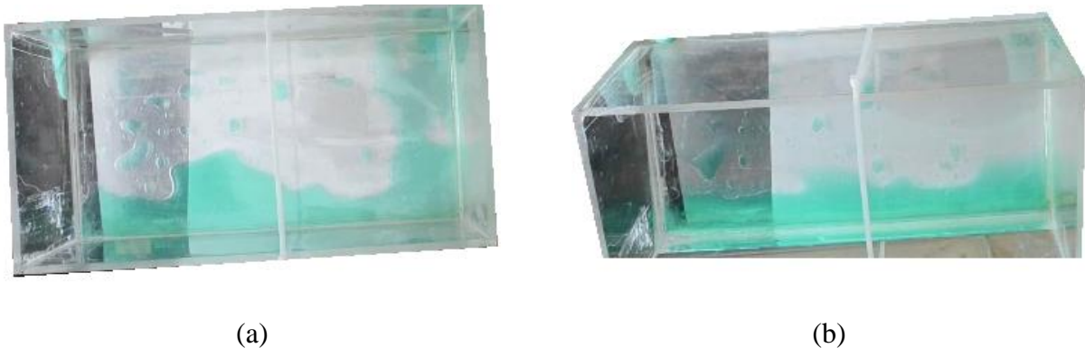
Figure 43. (a) Top view of water (colored green) in dispersed in kerosene (less than 5^\circ ). (b) Top view of water (greater than 5^\circ ).
