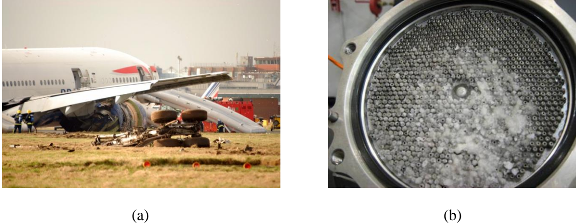
Figure 1. (a) The crash site at London Heathrow (Winter, 2010). (b) The formation of ice inside the heat exchanger (Haines, 2008).
