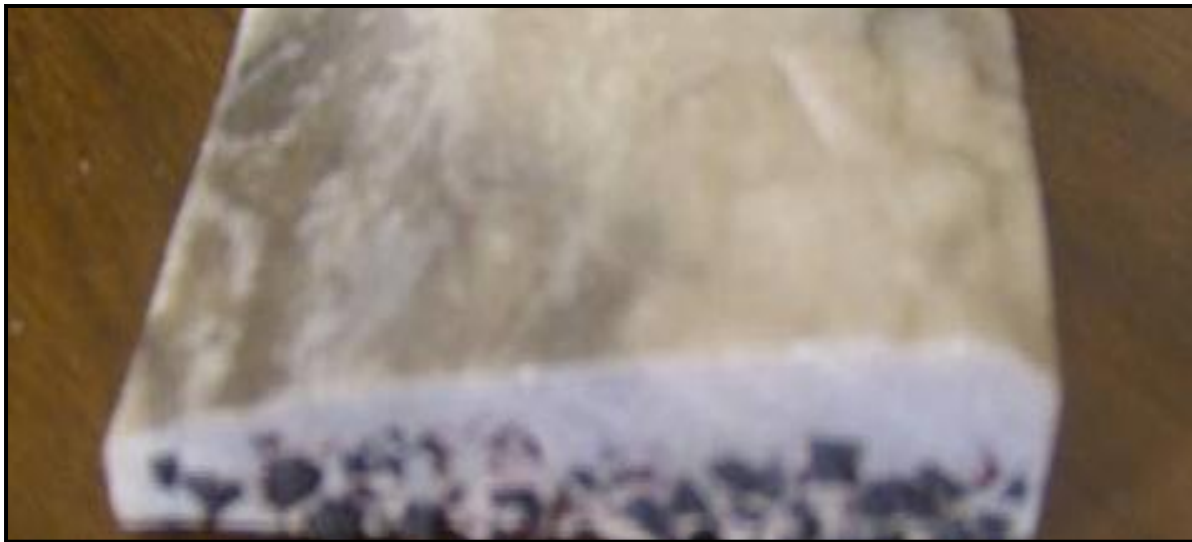
Figure 7.7. Cross section of stone cladding mixed with crumb rubber (Hamoush, et al., 2011).
