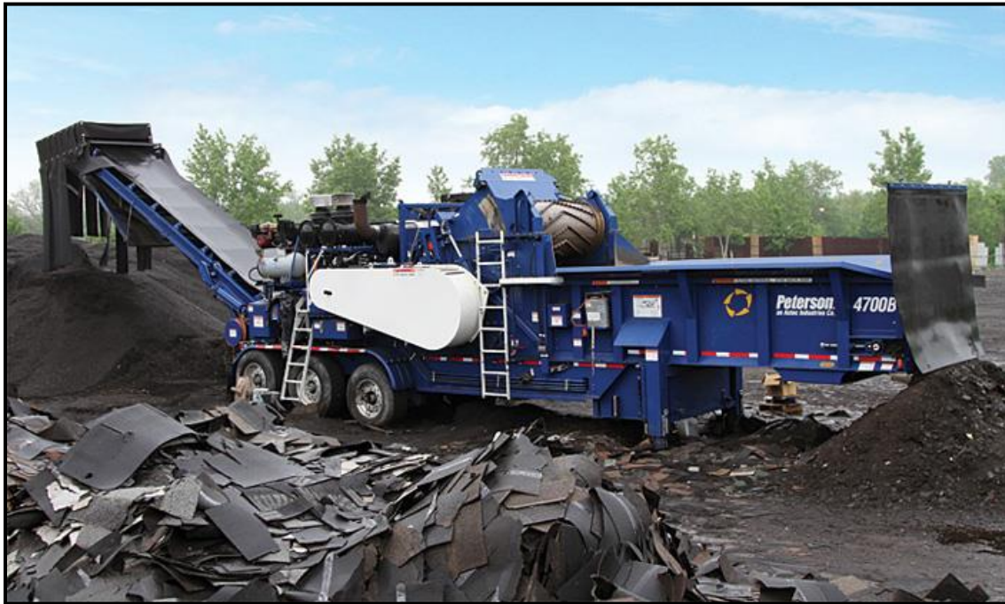
Figure 6.2. Roofing shingle grinding process in Texas (petersoncorp.com).
