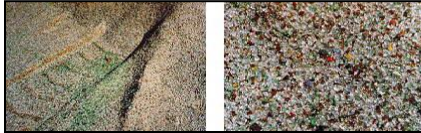
Figure 6.4. Glass for use in asphalt pavement (Schroeder, 2011).
