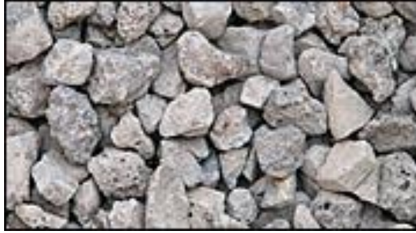
Figure 5.10. Air cooled coarse aggregate ((NSA), 2009).
