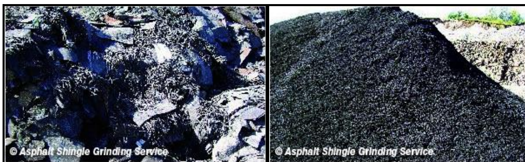
Figure 6.1. Roof shingle waste recycled and grinded (Asplat Shingle Grinding Service, 2012).
