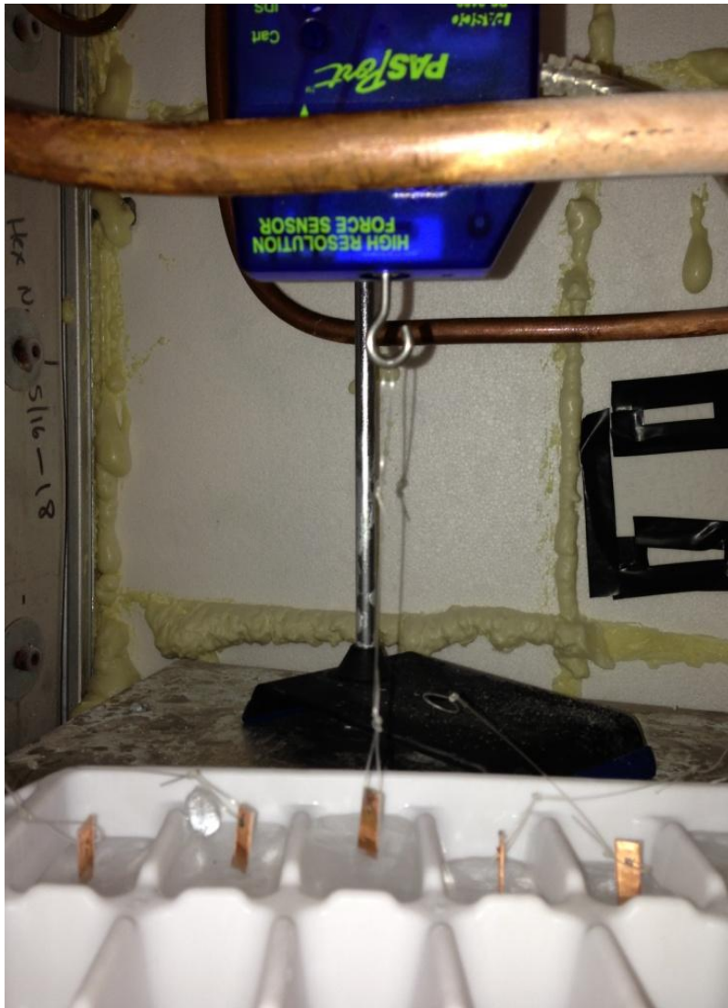
Figure 22. Experimental setup for the shear strength tests.
