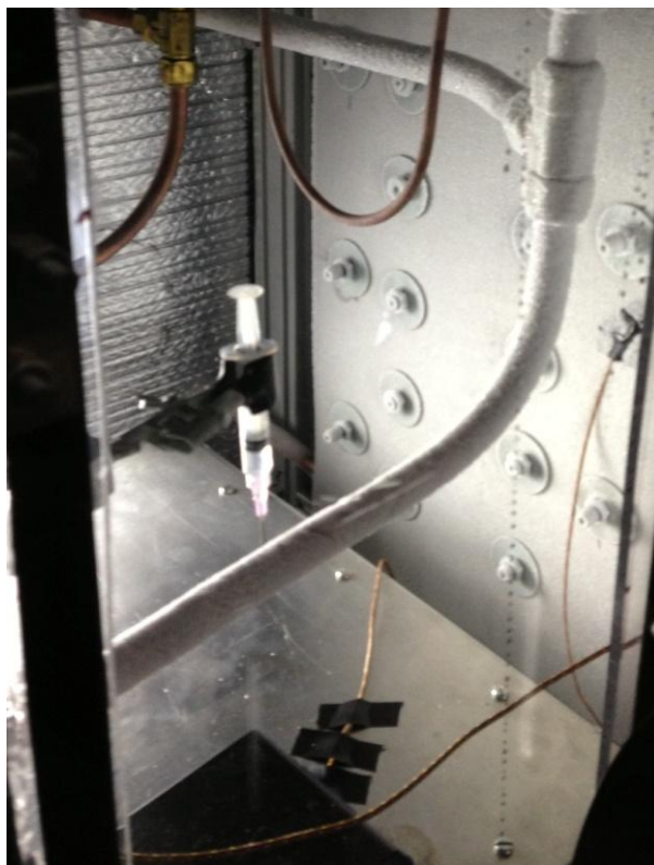
Figure 29. Experimental setup used to visualize freezing sessile droplets.
