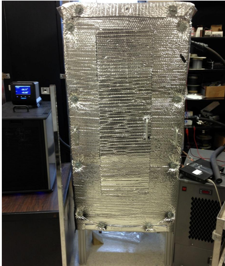
Figure 24. Environmental chamber used to simulate subcooled conditions.
